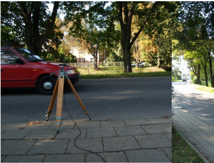
Figure 3 – Retroreflective sensor on tripod
